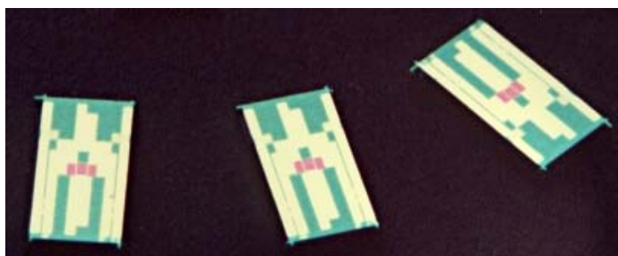
Figure 8 C2V Gas flowsensor chips and an SMD packaged flowsensor chip. The reddish rectangles in the middle of the chips are silicon nitride membranes, made with the help of wafer KOH wet anisotropic etching.
