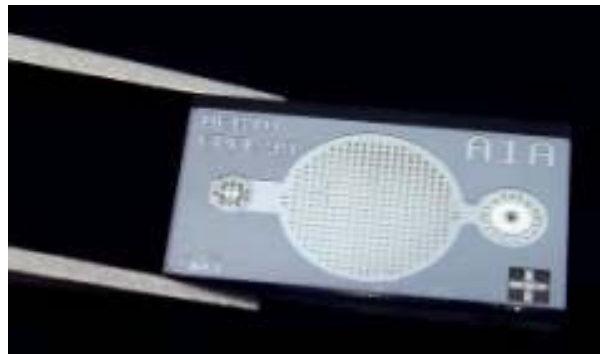
Figure 11A silicon micro pump, made from silicon and Pyrex glass, by Debiotech.
