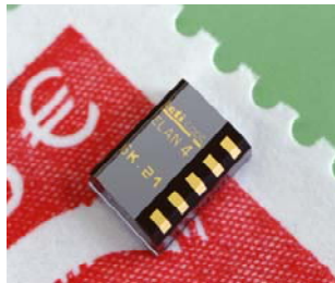
Figure 10. A Chip-size-packaged Twin-axis Accelerometer (Source: Tronics).
