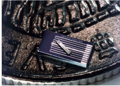
Figure 3. An Ultra-miniaturized Medical Pressure Sensor Chip just 0.1 mm x 0.14 mm x 1.3 mm (Source: Melvås P., Royal Institute of Technology, Sweden).
