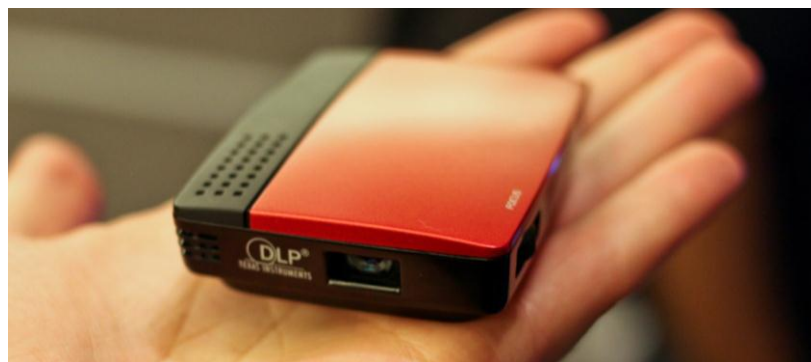
Figure MEMS9 TI's prototype USB picoprojector nHD Pico with 20 lumens, 640 x 360 resolution, a contrast ratio greater than 1,000:1, a true RGB LED wide color gamut and reliance on a low-power Pico DPP2601 2607 ASIC processor.
