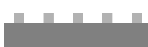
Etch hardmask and strip second resist
