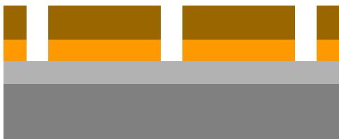
Print trenches and etch hardmask
