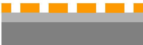
Etch hardmask and strip second resist
